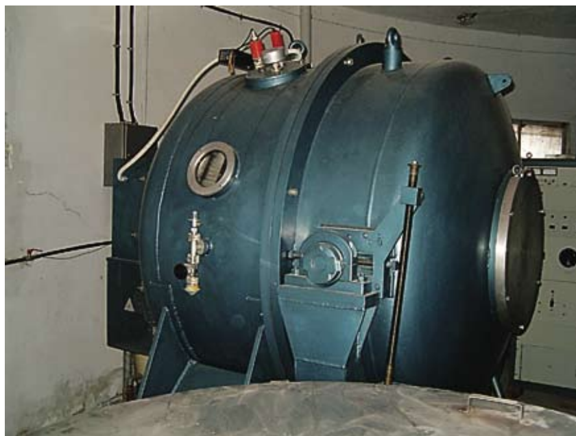
Figure 3. The aluminizing plant unit at Kryoneri Observatory.
