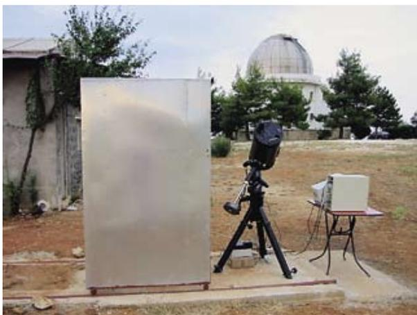
**Figure 2.** The CELESTRON telescope and PC driving the “seeing” measurements, next to the small enclosure built to protect the telescope from weather. At the background, the 1.2m telescope dome of the Kryonerion Observatory can be seen.
