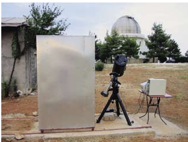
Figure 2. The CELESTRON telescope and PC driving the “seeing” measurements, next to the small enclosure built to protect the telescope from weather. At the background, the 1.2m telescope dome of the Kryonerion Observatory can be seen.
